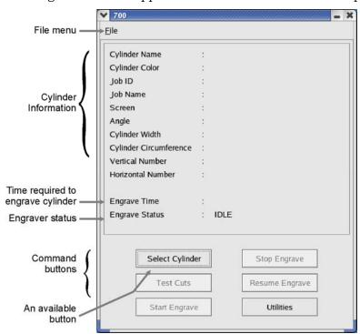
**Note:** One RTI computer can support multiple engraving channels. For example, you could have one dual-head engraver or two single-head engravers. A separate Engrave window is used for each engraver (or engraving channel) configured to your RTI.
