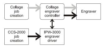
"Pass-through engraving" means that a CCS job must pass through the Collage RTI (engraver controller) to the engraver. After Collage has been integrated into your network, the Collage RTI—*not* the IPW-3000—actually controls the engraver.
